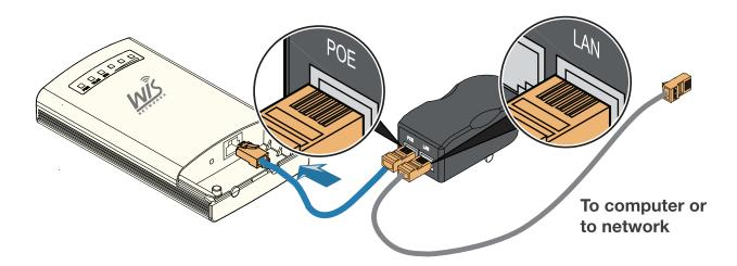
Connect one end of an Ethernet cable to the POE port of the provided PoE DC Adapter and the other end of the Ethernet cable to the RJ45 port of the device. Then, connect the LAN port of the PoE DC Adapter to a PC or switch using another Ethernet cable. Finally, plug the PoE DC Adapter into a standard electrical wall socket.
